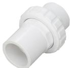
*The Plumbing Unions connect the plumbing lines to the components. Unions can become loose in transit and when seasons change. During the initial installation and each time you drain your spa, you should hand tighten all plumbing unions. The main cause of leaks inside the spa cabinet is plumbing unions that need to be tightened or seals that need to be re seated or replaced. Do not use tools or overtighten plumbing unions.*
